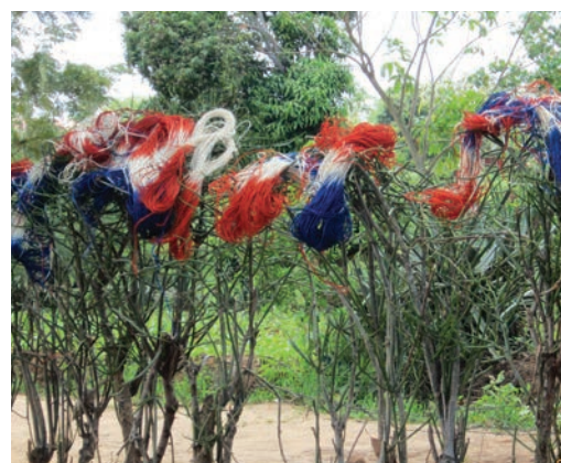
Small batches, unclean water, open fire, and sun-drying all undermine color control.
